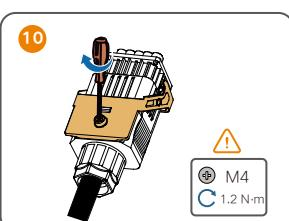
For inverter models  $\geq 15\text{ kW}$
